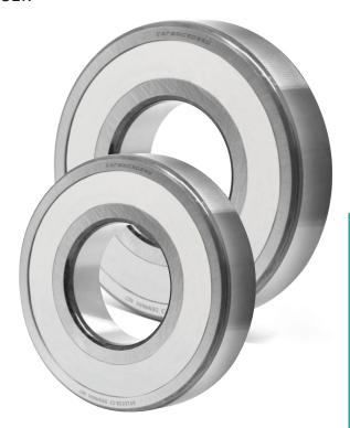
CeramicSpeed SLT is a polymer matrix saturated with lubrication oil. The matrix secure to retain oil right on the functional surfaces of the bearing under even very harsh conditions while at the same time preventing moist and foreign particles in entering the bearing.
